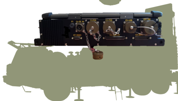
X500 with bottom box extension with integrated Arinc interface customized MIL-Connector rear box and external rugged 10" display with touch screen
